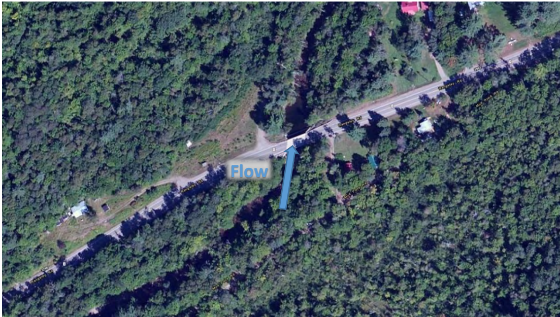
Figure 2. Air photo of bridge crossing showing scour hole downstream. Note skew of bridge structure to direction of flow.
